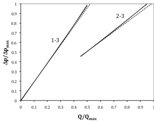
Figure 10 represents the linearization errors achieved with this arrangement. The maximum non-linearity error is of 0.12%. Obviously the Poiseuille relation is not used here for the reasons explained above.
