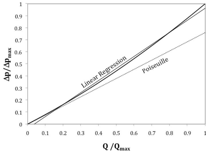
Figure 4 represents the errors achieved when these linear approximations are used as response. Obviously the linear regression performs much better than the Poiseuille approximation except at very low flow rates. In order to reduce these errors, Siev [3] recommends the use of a minimum value of 0.3 for  $L/(ReD)$ , and preferably of 0.6 or greater, so that the entry length errors become negligible.
