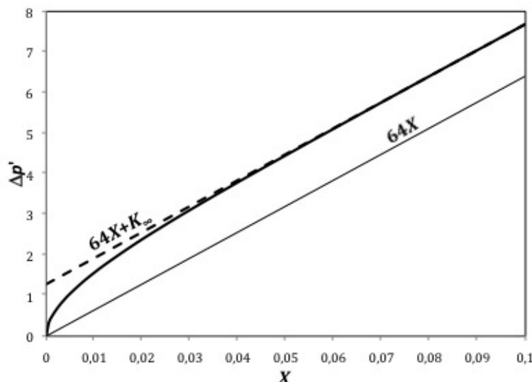
According to White [7], it can be considered that  $K$  approaches its final value  $K_\infty$  when  $X \approx 0.08$ . Ideally, and in order to obtain perfectly linear measurements, the pressure drop should be measured between pressure taps located at  $X > 0.08$ . Taking into account that we are seeking to use pipes of few millimetres in diameter this limitation would lead to laminar flow elements being very long.
