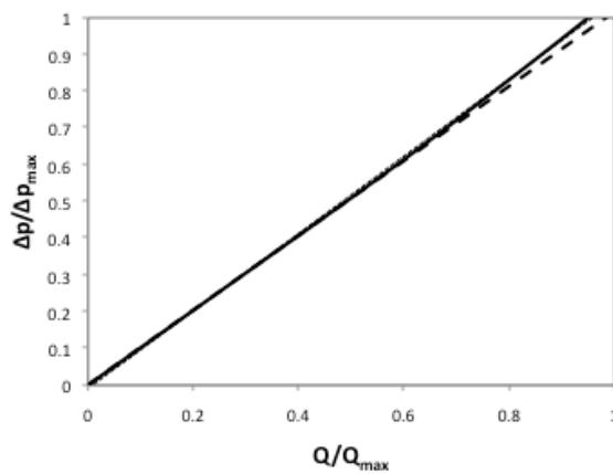
In the present case the coordinate  $x_1$  has been placed such that  $x_1/L = 0.14$ . The corresponding linearization errors are shown in Figure 7. Notice that the Poiseuille model produces negligible errors until the entrance length reaches position  $x_1$ , in addition its maximum value is now one sixth of the original one. On the other hand, the linear regression error has decreased by one order of magnitude.
