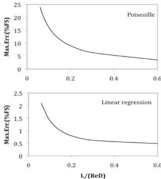
In the case of measuring the pressure drop between two pressure taps on the pipe wall; one at position  $x_1$  downstream the entrance and the other at the pipe end, the response curve of Figure 3 should change as in Figure 6.
