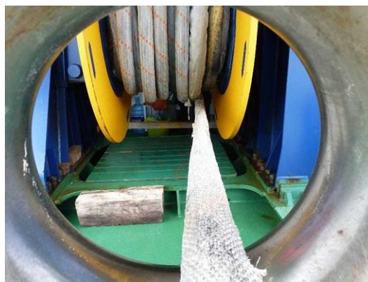
Fig. 15 – Fairlead on vessel, at the tow winch outlet.
