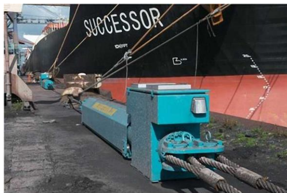
Fig. 12 – Hydraulic mooring system. Source: KRVE (2016)
